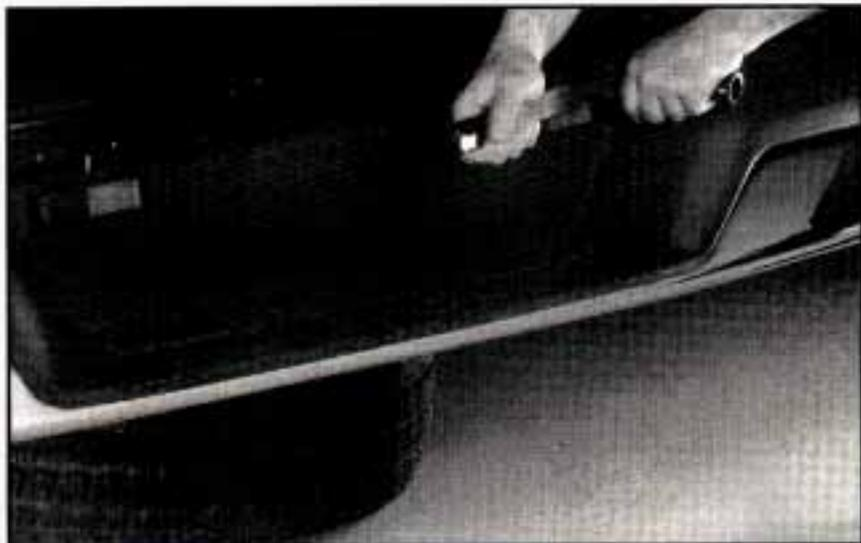
5. Put the flat end of the extension on an angle through the hole in the rear door frame, above the bumper. Turn the ratchet to the right until the tire is against the underside of the vehicle.
