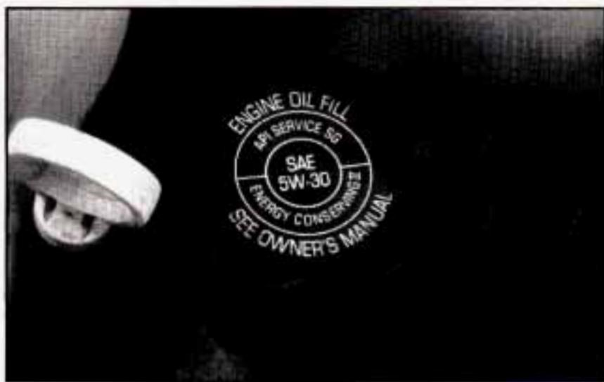
The engine oil filler cap is located between the coolant recovery tank and the air cleaner.
