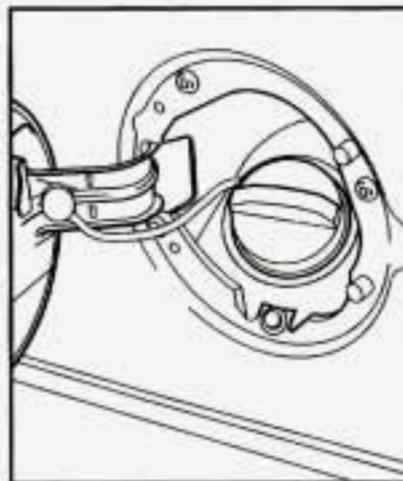
The fuel cap is behind a hinged door on the driver's side of your vehicle.
