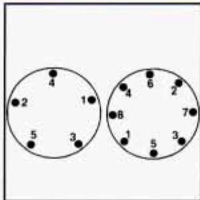
10. Tighten the nuts firmly in a crisscross sequence as shown. Rotate the wheel wrench to the right.
