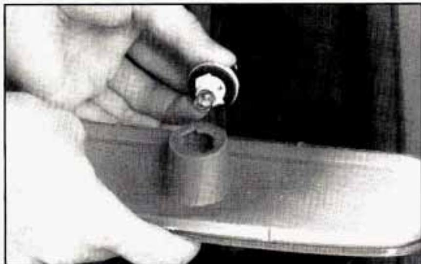
2. Unclip the bottom of the lamp from the grille.
