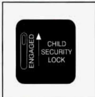
Move the button up to engage the security feature. Move the button down to return the door locks to normal operation.
