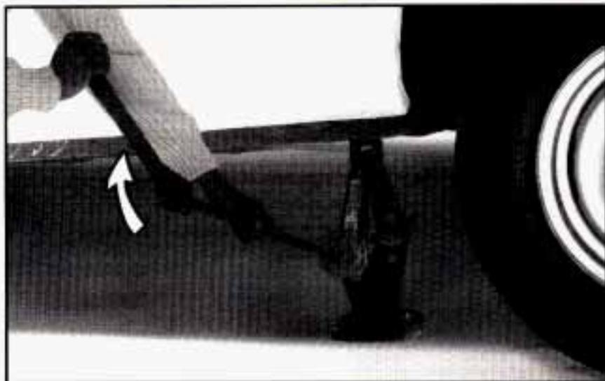
5. Raise the vehicle by rotating the ratchet to the right. Make sure the UP mark faces you. Raise the vehicle far enough off the ground so there is enough room for the spare tire to fit.
