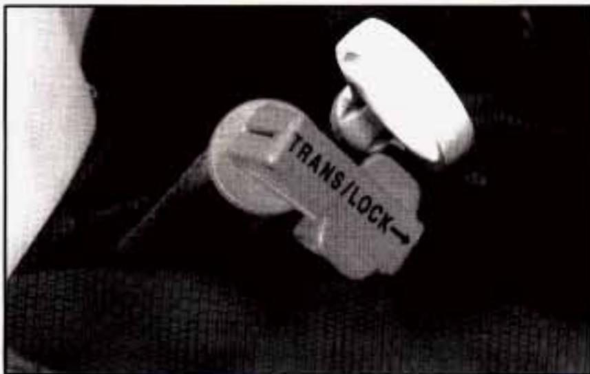
1. The transmission dipstick has a red handle and is located near the center of the engine compartment. Flip the handle up and then pull out the dipstick and wipe it with a clean rag or paper towel.
