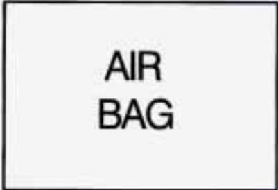
A rectangular box containing the text "AIR BAG" in a bold, sans-serif font, representing the symbol for the air bag readiness light on a vehicle's instrument panel.
