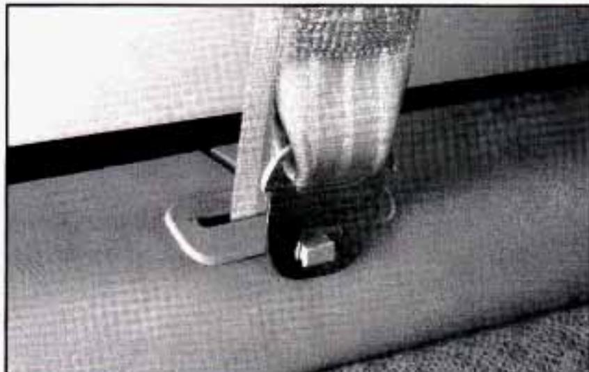
For the remaining rear seats, stow the safety belt latch plate on the clip at the window trim.
