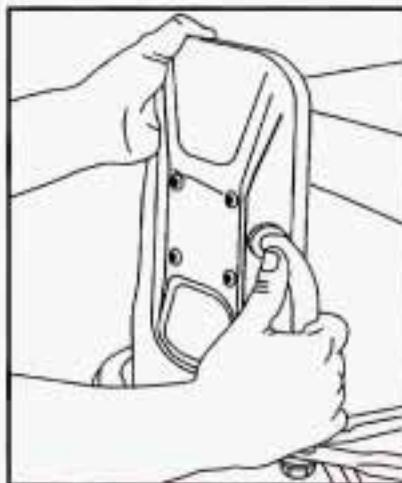
1. To adjust the mirrors when towing a trailer, rotate the mirror by pushing the mirror head toward the front of the vehicle.
