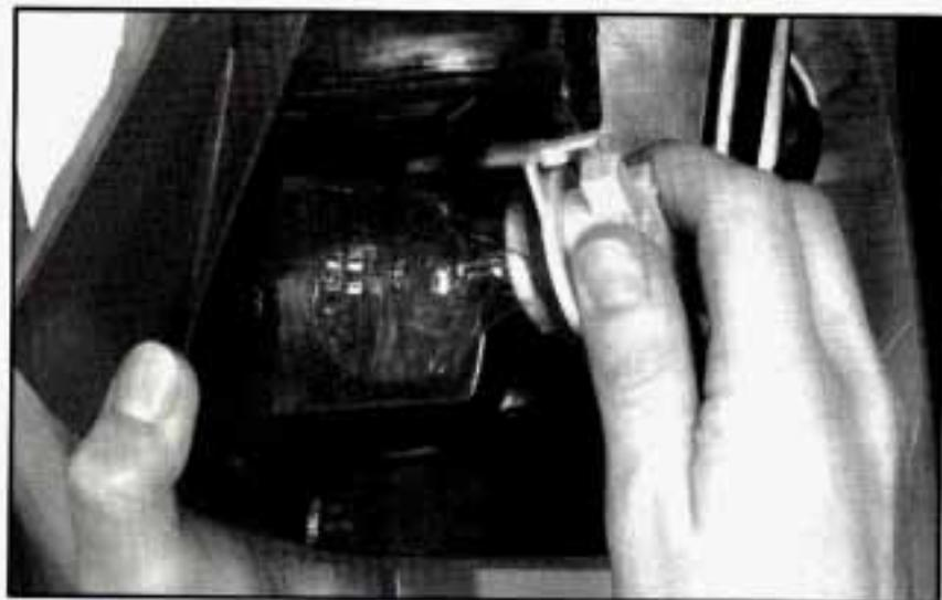
7. Turn the bulb to the left to remove it. Install the new bulb.
