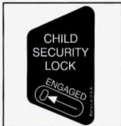
Move the button to the left to engage the security feature. Move the button to the right to return the door locks to normal operation.
