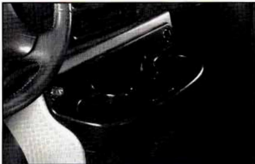
Your front storage compartment is at the center of the instrument panel extension, by the floor. To open the compartment, press down on inside portion of the handle and the compartment will open automatically.
